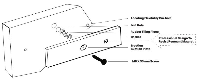
Attention : Don't screw too tight the suction plate. Keep proper flexibility for the rubber filling piece, to automatically adjust the suction force of the traction plate to the correct position.
